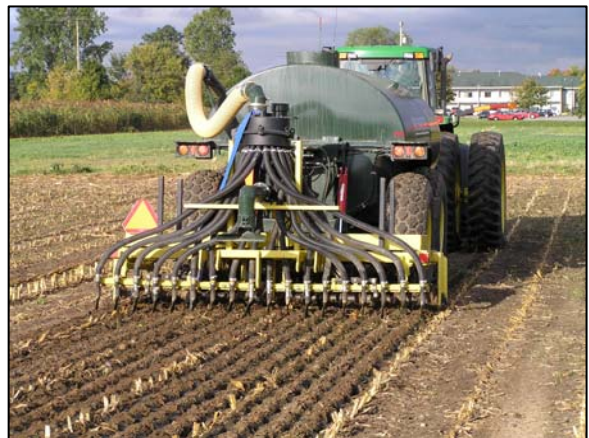
Figure 1. Excellent wheat and cereal rye cover crops were obtained by combining low-disturbance aeration tillage, seeding and slurry application in one efficient operation.
